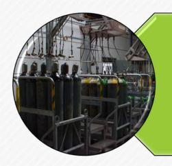
1980's introduction of: bespoke semi-auto filling (pressure temperature compensation); 200 & 230 bar; pallet filling; balanced valves; still limited factory build; still bespoke projects; manual information recording; high maintenance costs
